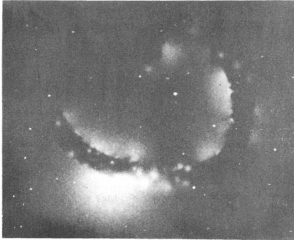
Figure 12. Autoradiograph of a deuterated Ti chip showing tritium-containing hot spots. (From Kaushik et al.93)
