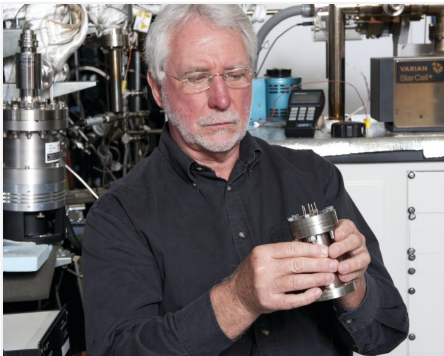
In a photo from 2012, Michael McKubre, one of the original cold fusion researchers, inspects a component of SRI International's Micromass 5400 mass spectrometer, an instrument dedicated to measuring ^3\text{He} and ^4\text{He} produced in palladium-deuterium and palladium-hydrogen LENR.
