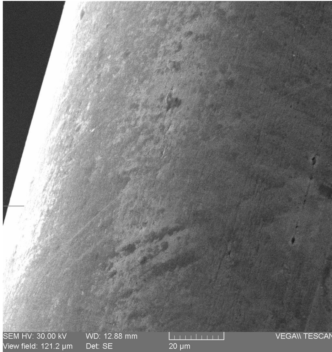
SEM. Details of wires after plastic removal: almost smooth surfaces.
