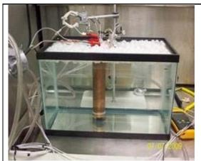
A new "calorimeter," shown immersed in this water bath, provides the first inexpensive means of identifying the hallmark of cold fusion reactions: the production of excess heat. *Credit: Melvin Miles*
