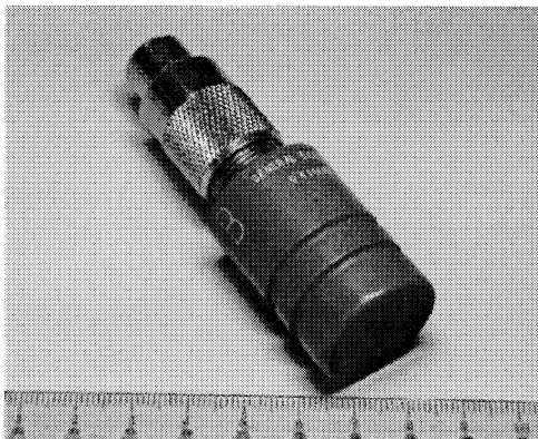
Fig. 5: Single element focused transducer used in this study (General Electric type B)
