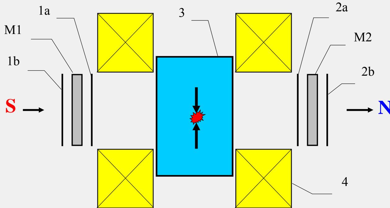
1 and 2 – X-ray photoplates, M1 and M2 – the material investigated. 3 – the thin wall plastic vessel, 4 – Helmholtz induction coils.  $S \rightarrow N$  – direction of magnetic field.
