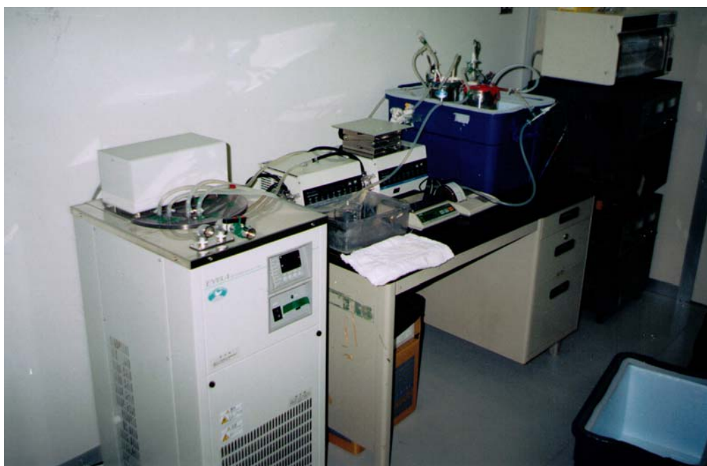
Fig. 2.4,2 The cells are inside Dewars. Cooling water is provided by constant displacement pumps to the left. Current, voltage, and temperature readings are recorded by electronics to the right.
