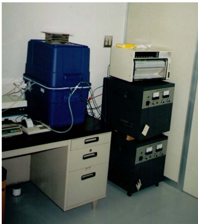
Fig. 2.4,1 Two electrolysis cells using DS-cathodes monitored by water flow calorimeters are inside a styrofoam insulation box. The cells have been operating during ICCF8 conference.
