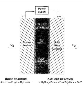
Anode and Cathade Reactions Produce gaseous oxygen and hydrogen, respectively. A power supply removes electrons from the porous anode and supplies then to the solid-metal cathode. The aqueous electrolyte between the electrodes completes the circuit by carrying (OH<sup>¬</sup>) to the anode.
